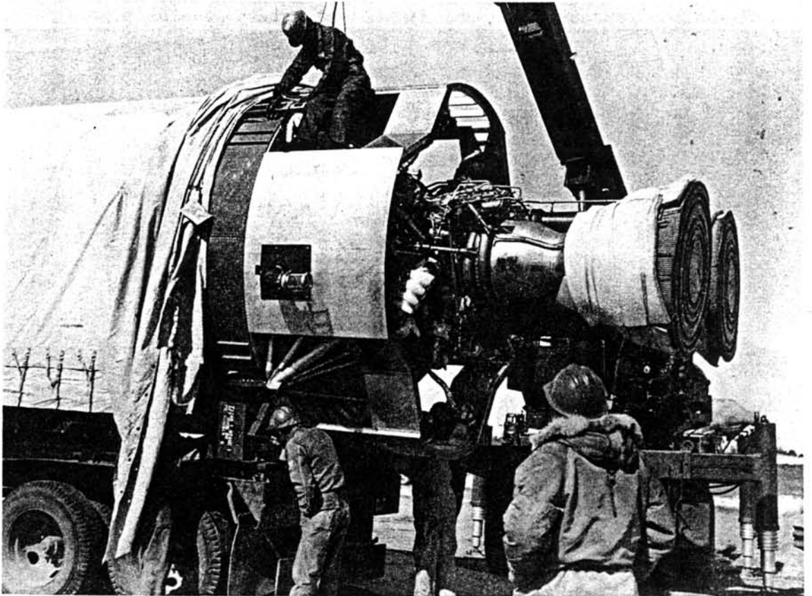
A TITAN I ICBM BEING PLACED ON TRAILER DURING DEACTIVATION AT LOWRY AFB, COLORADO.
